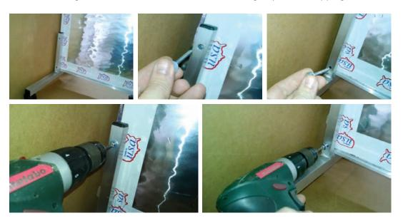
**4** Carefully tip the mirror and stand on its side, showing the bottom of the bumper bar. Drill drive the #8-18 flat head screws in the countersunk holes on bumper bar. Do not over tighten or strip. Set clutch on drill half the full strength setting.
